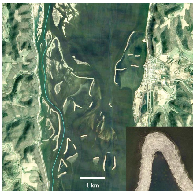
Figure 15. Satellite image (2021) of artificial islands created in the Mississippi River near Stoddard, Wisconsin, to enhance duck and turtle habitat. The inset (lower right) shows detail of the upstream end of one of the structures in the lower left of the main image.
